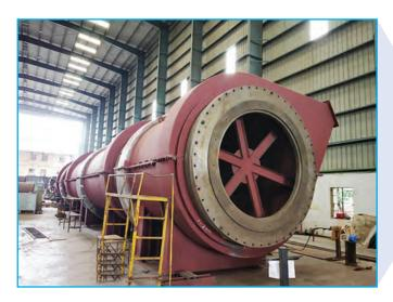
HF Kiln with Heating Jacket for M/s. TANFAC Industries Ltd. ready for dispatch
