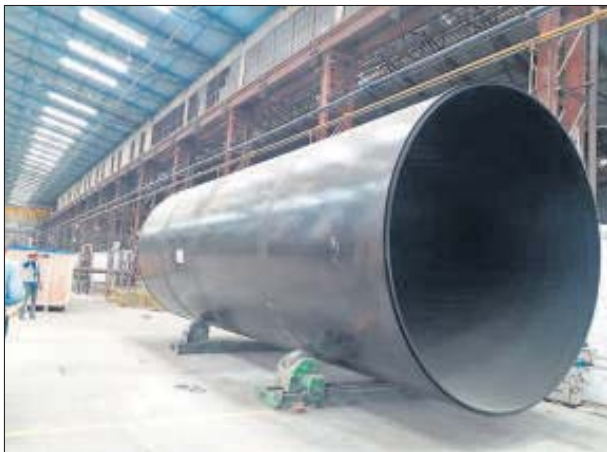
■ First-stage booster and flex nozzle control tanks were manufactured at Walchandnagar Industries Ltd. HT PHOTO
