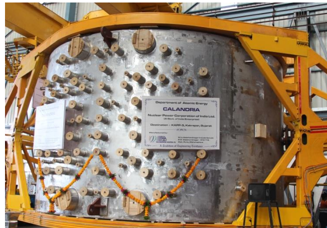
Calandria for 700MWe Nuclear power plant
